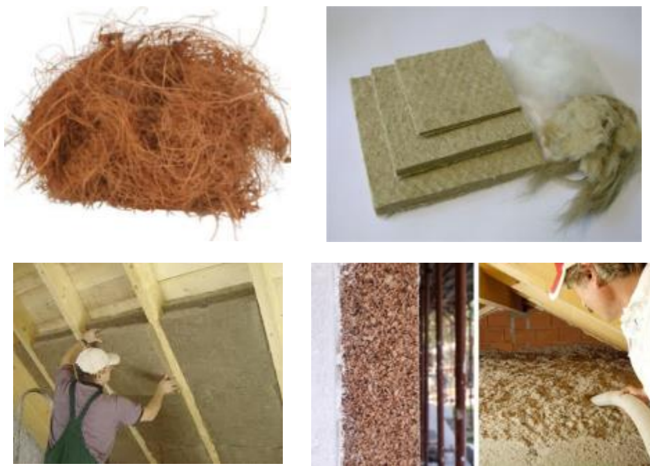
Figure 1: Insulation products in Flax Fibres, made from organically grown plants, non-polluting and of low energy demand, totally recyclable, biodegradable and compostable, durable and lightweight. They are characterized by their high stiffness, for the ability to attenuate vibrations and for low density compared to other fibres. They are excellent thermal and acoustic insulation materials,, eco-friendly and with a low wear level. Flax Fibres can be used to insulate roofs, floors and to create ventilated roofs and ventilated coats.
