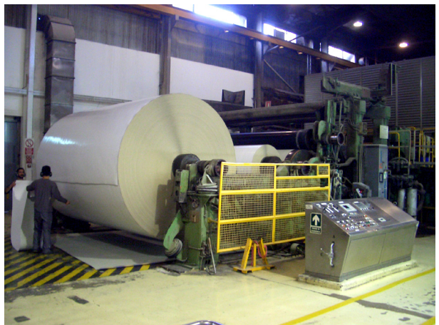
First board reel produced at Barcelona Mill with hazelnut shells in the middle layer
