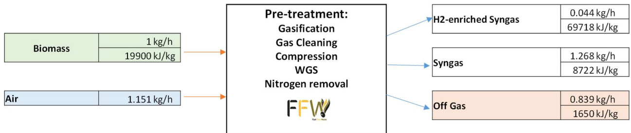
Figure 25. Base case mass balance scheme (chemical pre-treatment)
