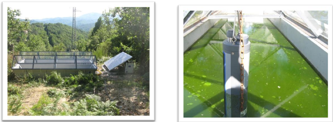
Figure 5 Open photobioreactor (pond)
