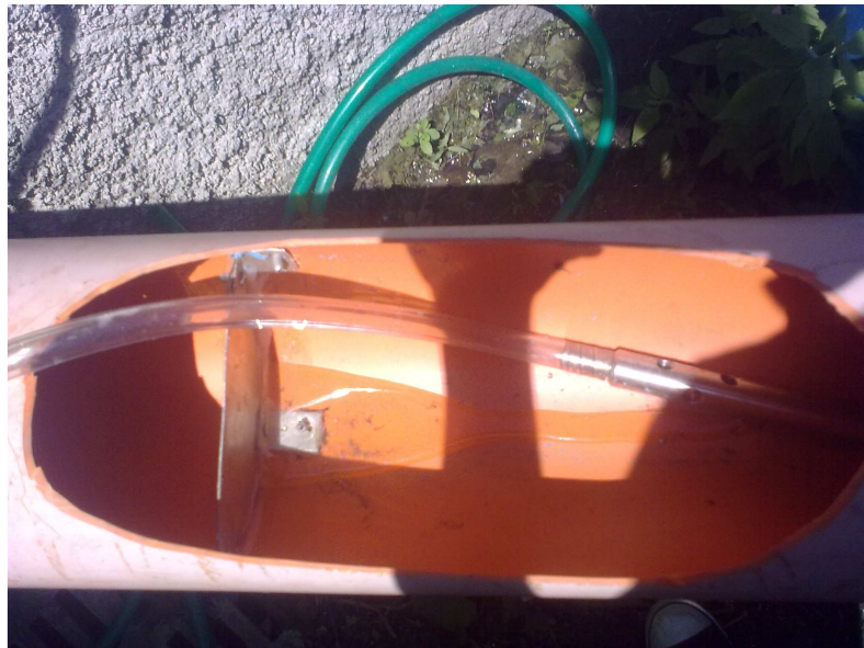
Fig. 20: particular of the rectangular weir for the submergence of the intake probe
