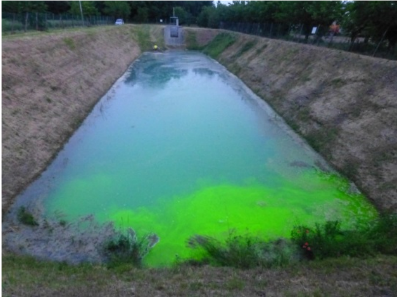
Figure 3 – Injection of Fluorescein in the Mereto Infiltration Pond.
