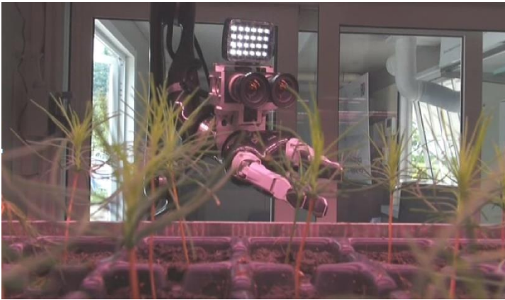
Figure IX: The robotic arm with the stereo camera and the gripper
